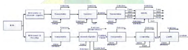
Figure 46. Waste management scenario: Waste is pre-treated and pre-sorted into biodegradable and non-biodegradable material for further anaerobic digestion and composting. Residues end in landfill. Plastic, paper and ferrous material are recycled.
