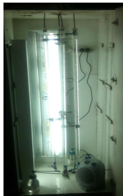
Figure 50. The photo-bioreactors within the temperature controlled cabinet
