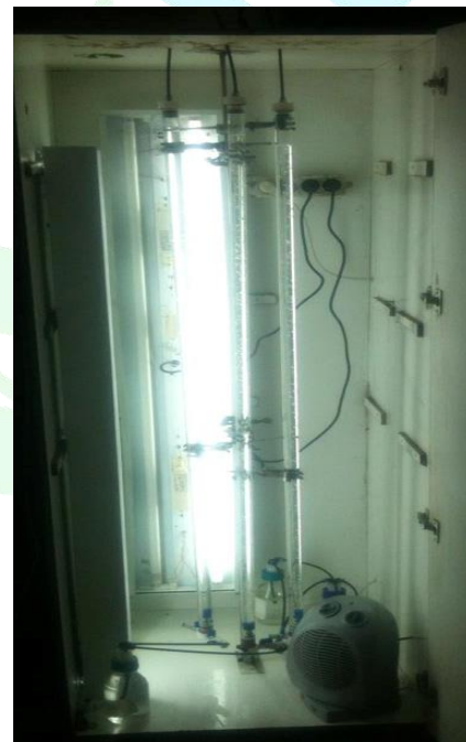
Figure 75. The photo-bioreactors within the temperature controlled cabinet
